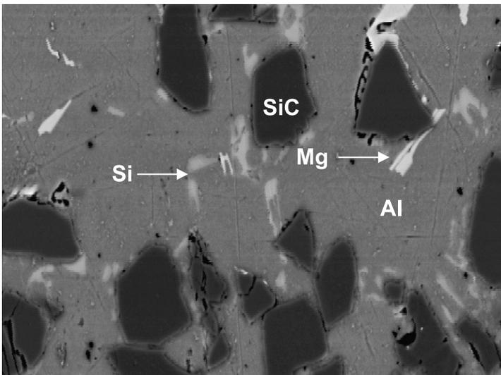
**Figure 1.** Microstructure of rolled 31% SiC in the as received condition showing four distinct phases: aluminium matrix, SiC particles, eutectic region of aluminium and silicon and Mg phase.
